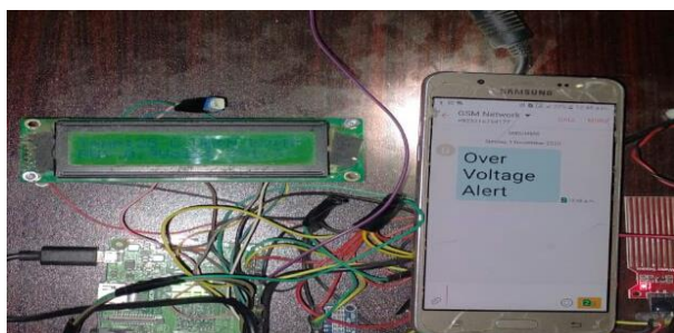
Fig. 8. Fault Due to Overvoltage
