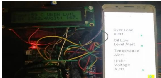
Fig. 11. Fault Due to temperature, overload, under voltage and low oil level
