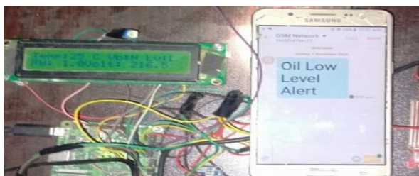
Fig. 9. Fault Due to Low Oil level
